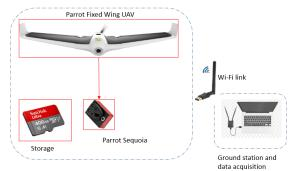
Overview of the multispectral imaging system with the UAV proposed.
