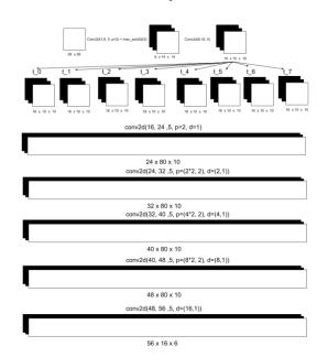
The Attention Neural Network (C-DATM) that controls pan-tilt-zoom cameras and has active hand-off capabilities
