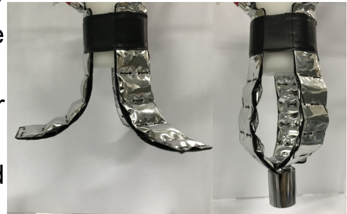
A gripper connected by soft pneumatic actuators
