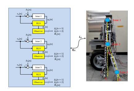
Fig. 1 Experimental setup for RLS-SOB control
